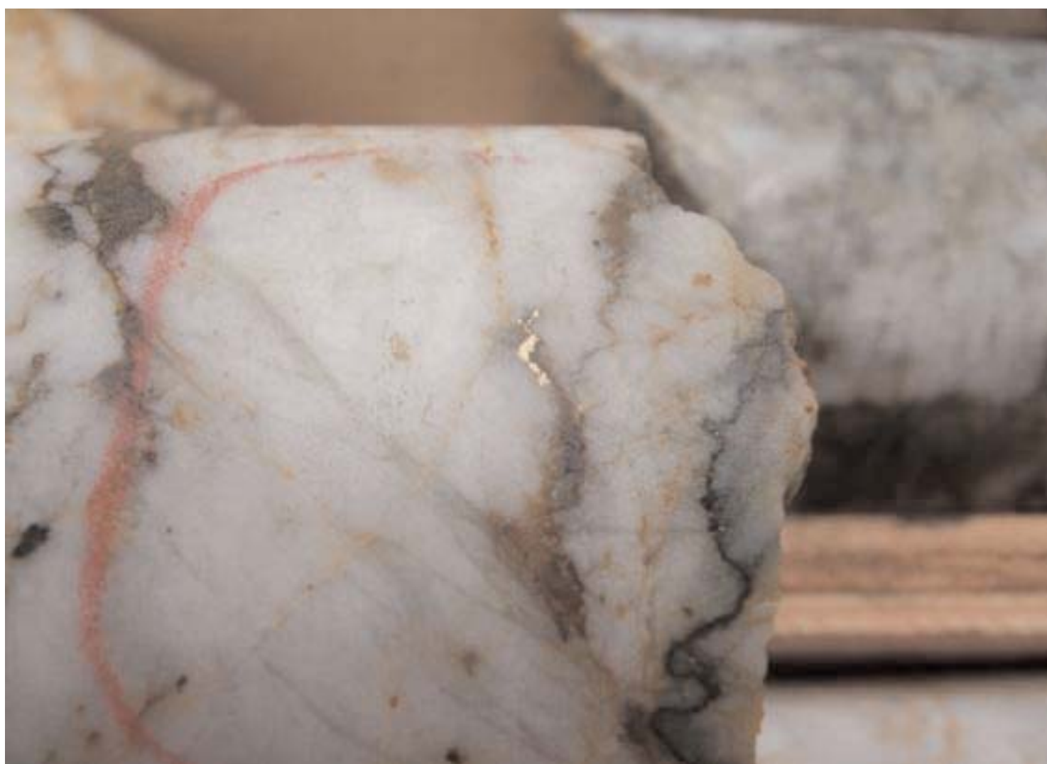
Figure 1 Drill core with visible gold, Elizabeth, 2007 exploration program
